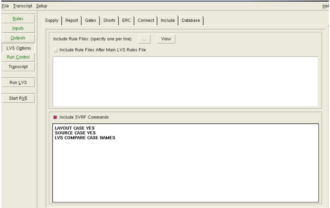
7. Go to Supply → And Type in the Power Nets and the Ground Nets. These need to match the power and ground pins in the schematic and the layout. In this example they are VDD and GND
